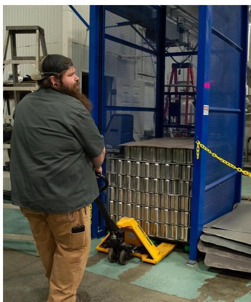
Jeffery is using a jacklift to take all of the empty, lidless cans and place them into the assembly machine. The machine will then lift the cans to the top where they will be brought down again so they can be filled and assembled.
