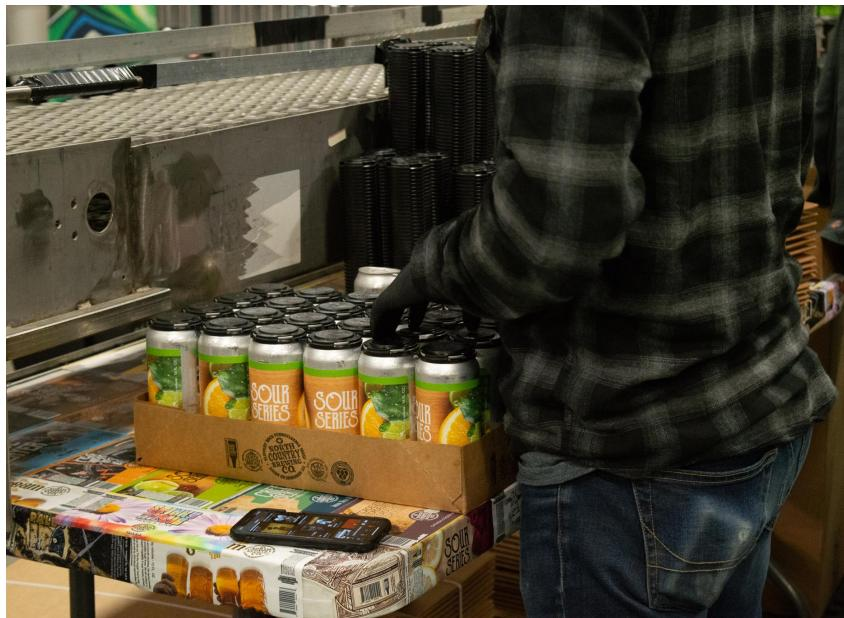
The cans are being taken off of the assembly line when finished where they are grouped together by fours with plastic pack rings that are added by hand. Next to Austin, who is packaging the beer, lays his cellphone which is playing Brockhampton over the speaker while he works.
