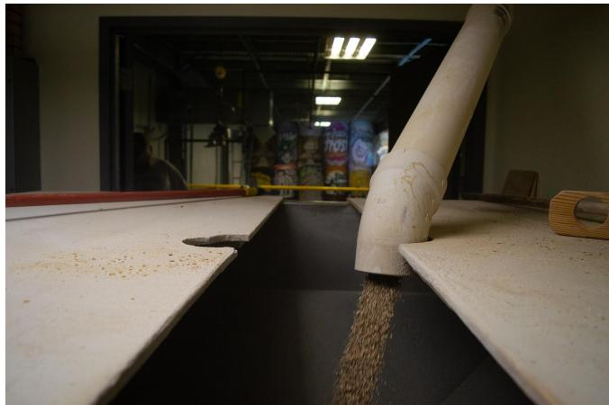
The grain falls from the chute and into the grist case so that it can be weighed and inspected. After the weigh in and inspection, it will go through another series of chutes and be gradually placed into the mash tun, where it will begin the mashing process.
