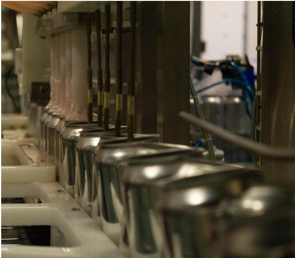
Empty cans are being filled with the Prickly Pear Sour, that holds a pink tint. They move through the assembly line, the rods holding them in place before being filled with the sour.
